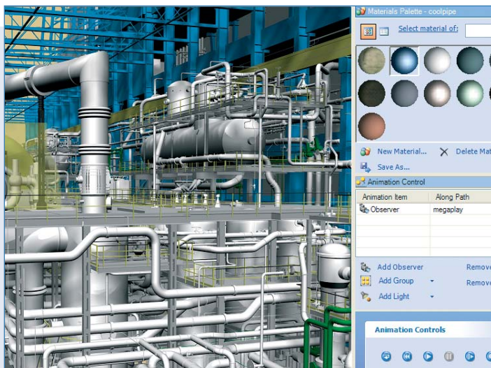
Material, texture and lighting controls for highly realistic visualisation Courtesy of Paks Nuclear Plant Company, Hungary
